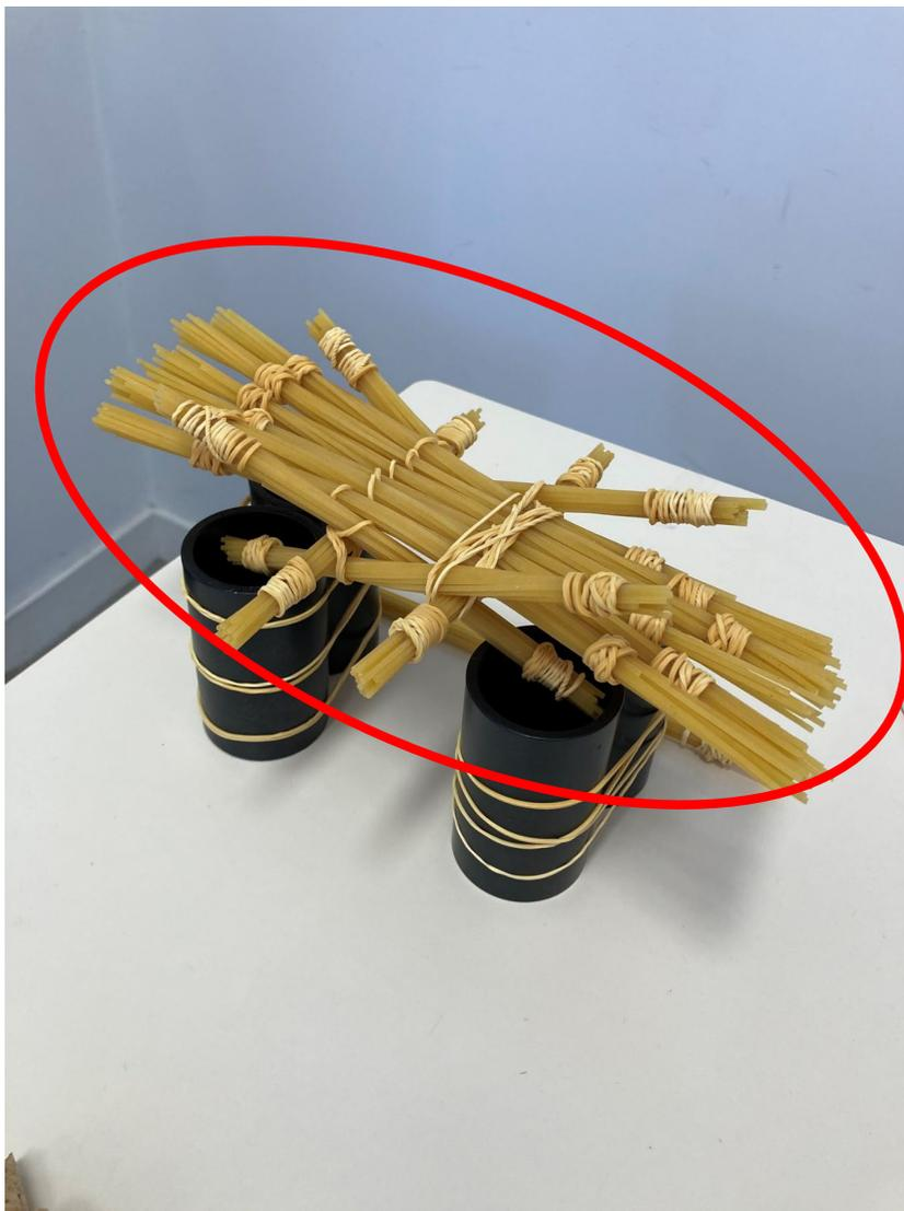
We used about 180 spaghetti and nearly 20 rubber band. The structure was able to hold 4 phones with ease, even though it bended a bit. That's why we put it on some cut pipes, attached also with rubber band, and that's how this work of art is born!
